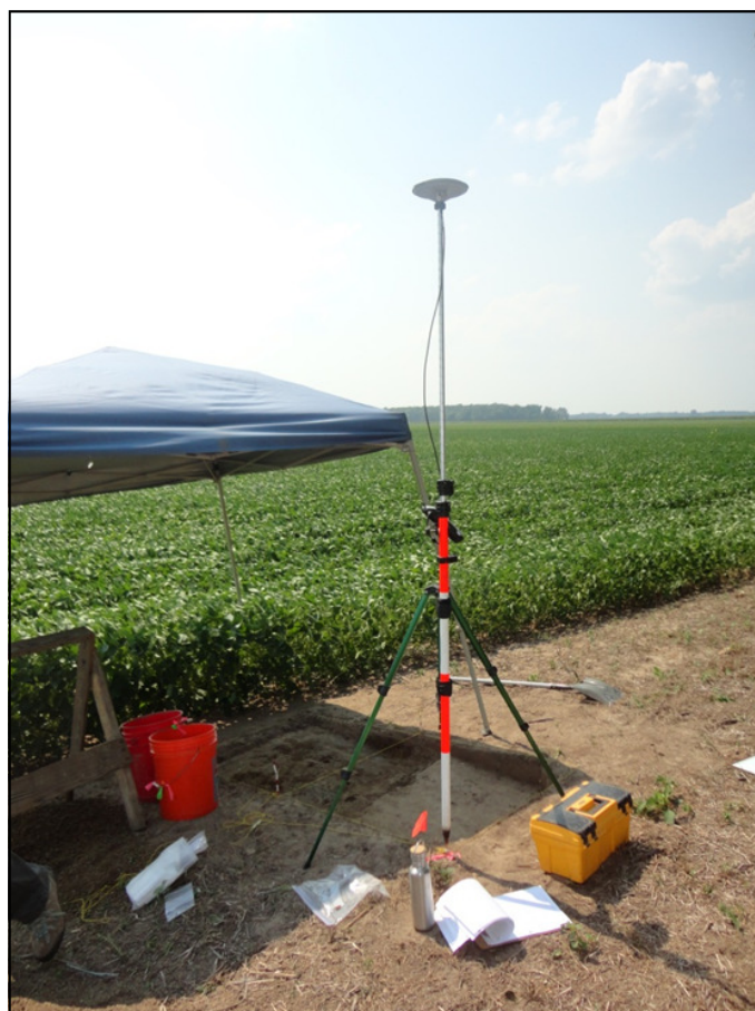
Figure 8. GPS unit set up over test unit corner
