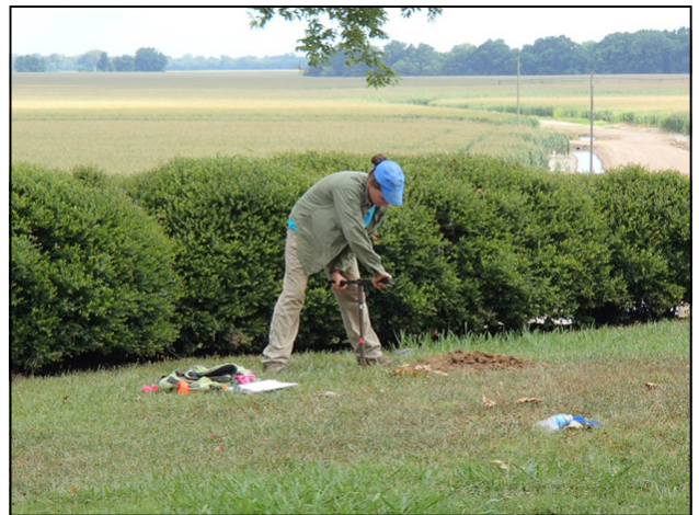
Figure 3. Augering with three inch bucket auger at Mt Helena
